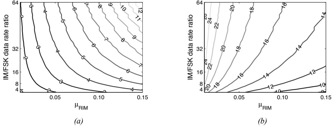
Figure 2. Optimum values of extinction ratio (a) and SIR (b). Both magnitudes are expressed in dB.
