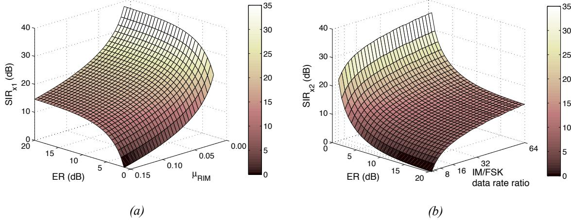
Figure 1. Signal to interference ratios of IM-modulated data (a) and FSK-modulated data (b).
